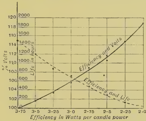
FIG. 194.—Curve of Relation between Efficiency and Life of Carbon Filament Glow-lamps.
