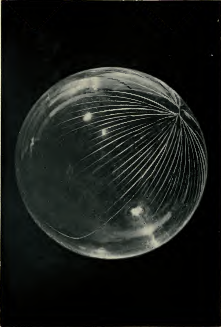
GLASS GLOBE CRACKED BY INTERNAL PRESSURE, ILLUSTRATING THE CAUSE OF THE BRIGHT STREAKS RADIATING FROM TYCHO.
