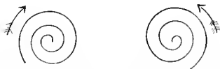
FIG. 5.—Diagram showing section of a vortex ring in its first stage. The arrows indicate the direction of the motion of the molecules (Hovenden).
