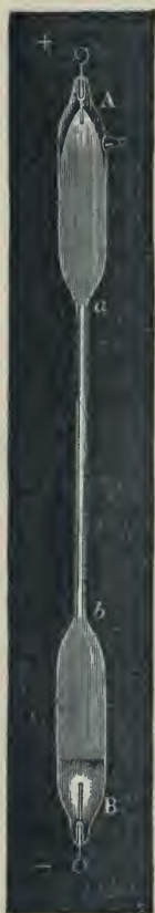
FIG. 27.—Geissler's tube, showing electric discharge.
