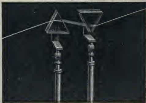
FIG. 10.—Recomposition of white light by means of a second prism.
