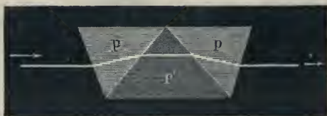
FIG. 18.—Direct-vision prism with three prisms, shewing path of ray.
