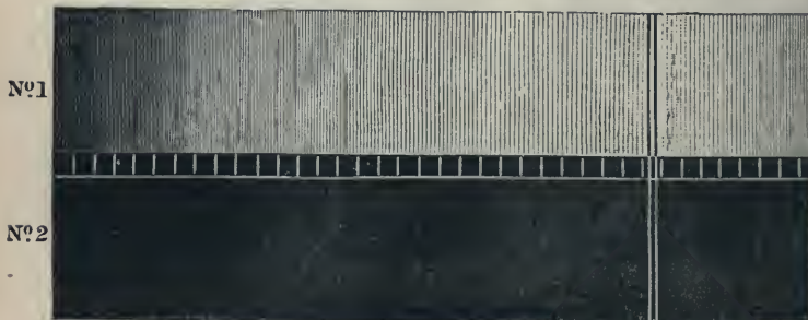
FIG. 51.—Coincidence between the bright line given out by sodium vapour and the dark line produced by the absorption of sodium vapour.
