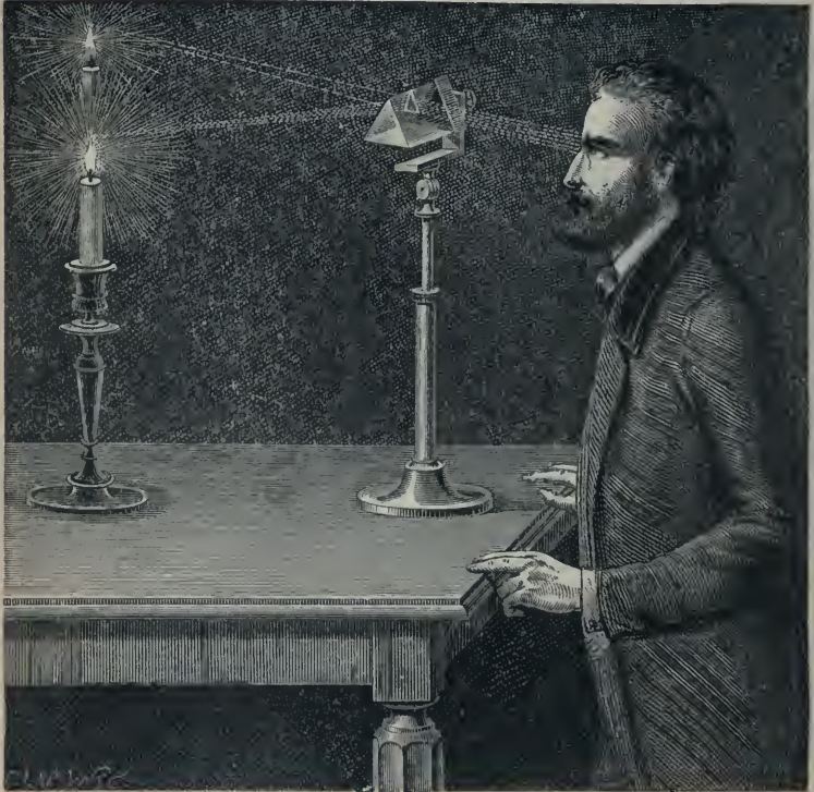
FIG. 8.—Images of objects seen through prisms.
