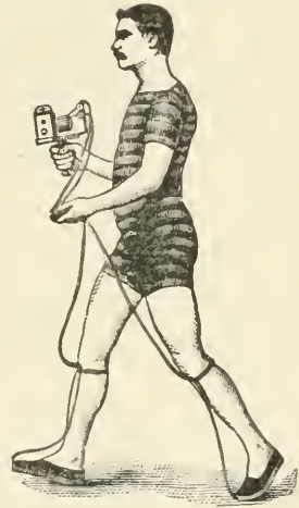
FIG. 32.—Walking with Pneumatic Shoes and Recording Drum.
