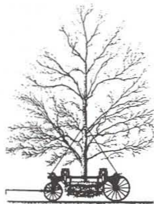
Manipulation of nature: "Tree moving Machine ... larger trees could be transplanted and the lag between planting and finished appearance reduced..."
