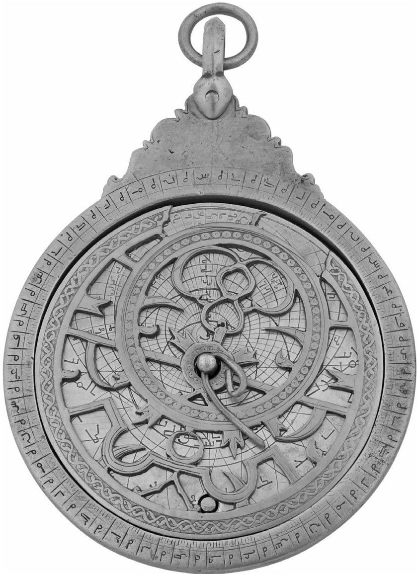
Figure 19.3. Fifteenth-century Eastern brass astrolabe body, Iran. Fake, identical tympan and symmetrically located, unnamed stars on rete. Courtesy of the Adler Planetarium, Chicago (A 91).
