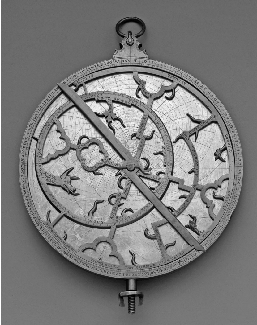
Figure 19.1. Mid-thirteenth-century English brass astrolabe with silvered plates or tympan. Courtesy of the Adler Planetarium, Chicago (M-26).
