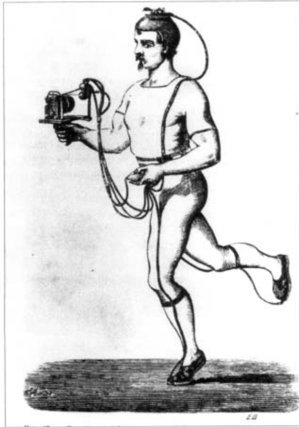
Runner with recording apparatus and pneumatic system inserted in his shoe.
