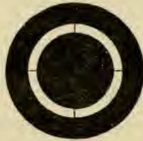
FIG. 45.—Diaphragm showing annulus, the breadth of which may be varied to suit the state of the air.
