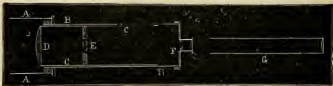
FIG. 46.—The annulus is viewed and brought to focus by looking through apertures in the side of the tubes. A, sliding eye-tube of telescope; B, tube screwing into eye-tube; C, tube sliding inside B, and carrying lens D and diaphragm E; F, lenses bringing image of diaphragm to a focus at the place generally occupied by the slit of the spectroscope; G, collimator of spectroscope.
