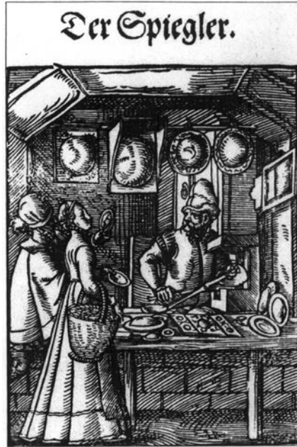
This 1568 German print of Der Spiegler (The Mirror-Maker) shows the craftsman cutting circular convex mirrors with special scissors while talking to customers.
