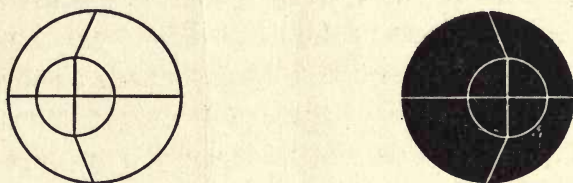
Fig. 69. — By combining these stereoscopically the effect of metallic lustre (similar to graphite in this case) is obtained.
