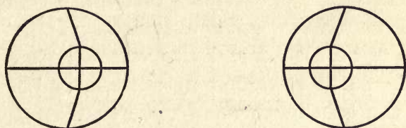
Fig. 2. — Stereoscopic pictures for combining by converging or diverging the optical axes.
